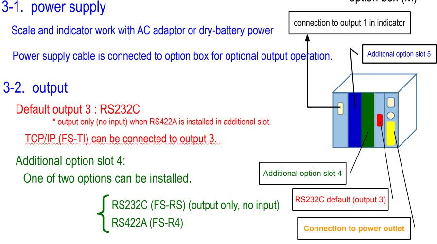
Additional option slot 5: Relay contact (FS-LM) can be installed here.
