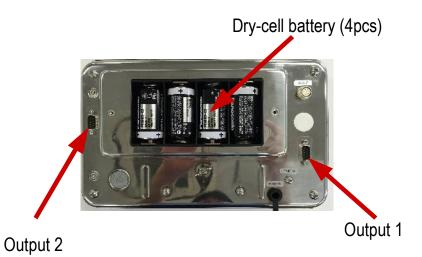
AC adaptor (parts code : UM117) Dry-cell battery (4pcs) available battery : D type (U.S.A), R20 and L20 (IEC catagory) continuous operation time FS 623 ~ FS 200K1G FS150K1GF & FS300K1GF Macklit OFF Backlit ON Backlit OFF Backlit ON alkaline 750 hours 300 hours 500 hours 250 hours
