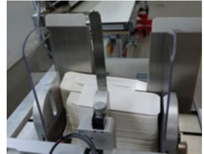
Stack processing of non erected cartons
