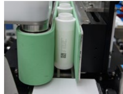
Application and serialisation of the labels
