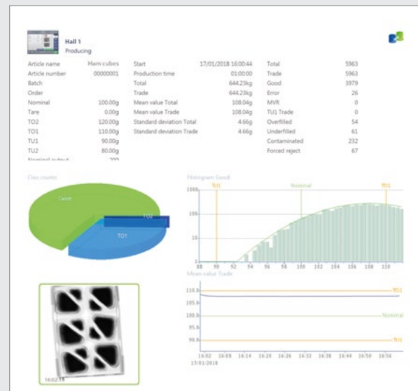
Production details of a machine with information on the mean, standard deviation and sorting limits.
