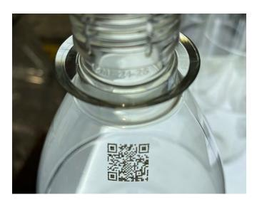
Laser marking is the method of choice to ensure that the coding on the bottle remains legible throughout its entire lifetime. The challenge lies in ensuring constant readability and avoiding damage to the plastic at the same time. The individual serial number is encoded in a QR code in compliance with the GS1 Digital Link Standard. Both industrial camera systems and smartphones are capable to read this code.
