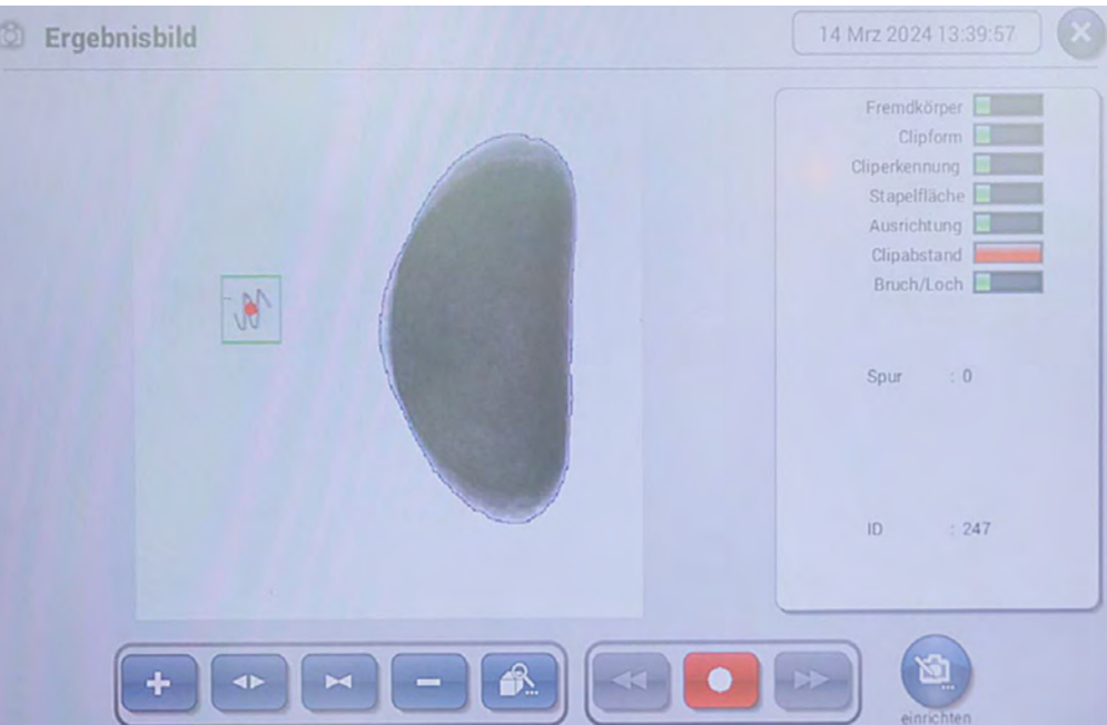
X-ray image of a pack of sliced bread with incorrect clip positioning
