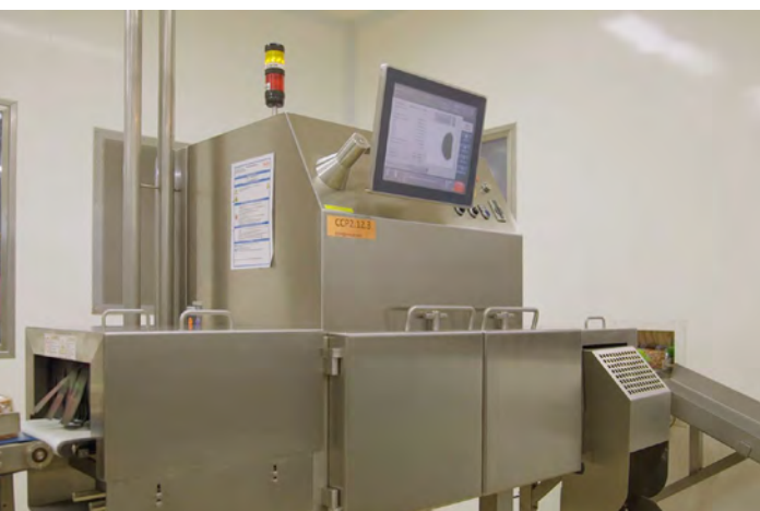
The SC-W combination solution: X-ray and weighing in a single system
