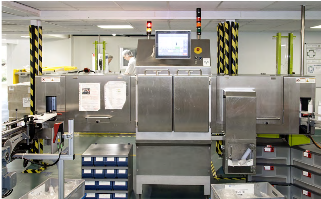
X-ray scanner at Laboratoire de la Mer. Adaptation by Wipotec to the specifications of Laboratoire de la Mer, with a single conveyor belt passing through the X-ray scanner, guarantees that unstable bottles are transported reliably and safely during inspection.
